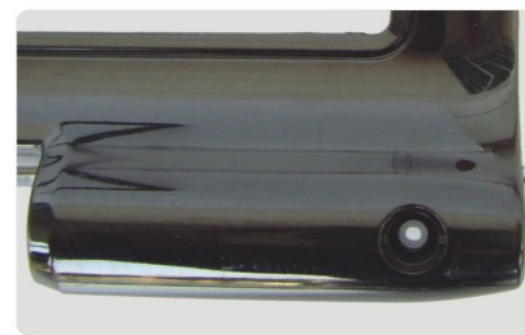
图 (2): 消除产品表面浮纤情况 (笔记本电脑机前壳) Fig (2): Eliminated fiber-mark on the product surface (Front-case of Notebook PC)
