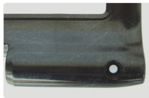
图 (1): 产品表面出现浮纤 (笔记本电脑机前壳) Fig (1): Fiber-mark on the product surface (Front-case of Notebook PC)
