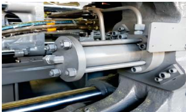
Optional item: Hydraulic ejector for special needs of core pulls / unscrew device
